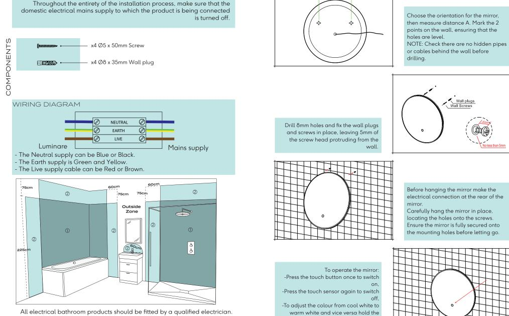
Before drilling, ensure there are no hidden cables or pipes in the wall.
