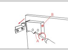
**60cm + models:** Locate the brackets on the furniture to the mounting plates on the wall. Secure the unit to the wall by tightening the nuts with a spanner.
