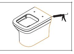
Add a consistent line of silicone sealant around the back of the pan, creating a watertight seal between the pan and the wall. Allow to cure for 24hr before wetting.
