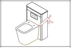
Having finished the installation of the cistern or flush plate/button, apply a later of silicone sealant between the Wc pan and BTW unit. This will ensure the unit is protected against any liquid damage.
