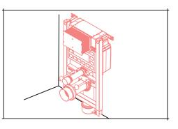
Before installation of the WC unit, the flush frame selected should be mounted on the desired locaton and all plumbing to the cistern frame should be done.
