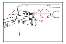
Locate the hangers onto the wall mounting plates.
