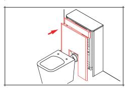
Secure the unit to the wall, by drilling the angle brackets to the inside of the side panels, as well as the back wall.
