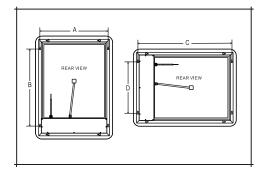
Measure distance A & B or C & D. Mark the 4 points on the wall, ensuring that the holes are level.
