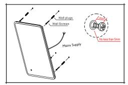
Drill holes and fix the wall plugs and screws in place, leaving 5mm of the screw head protruding from the wall.
