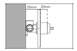
Ensure the valve is set back from the finished front face of the wall by the correct depth of min 55mm max 75mm (Allow for tiles, adhesive, etc).
