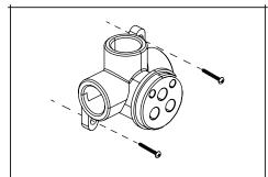
Fix the valve to the supporting framework using the screws provided.
