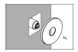
Remove the plastic cover protecting the chrome valve. Slide the chrome face plate over the valve until flush against the finished wall surface.
