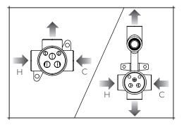
Ensure the pipework is correctly arranged to suit the position of the hot/cold inlets (etched on the valve body).
