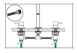
Screw the flexi pipes onto the bottom of the handle body and connect to the mains.
