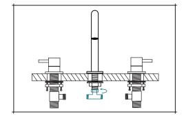
Screw the brass tee junction to the thread protruding from the spout.
