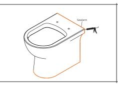
Add sealant around the back of the pan, creating a watertight seal between the pan and the wall.
