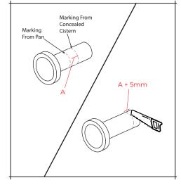
Place the Inlet and outlet pipes on the Wc pan and mark where they extend past the edges of the bowl. Then place the pipes completely onto the sanitary unit and mark them where they emerge from the unit.
