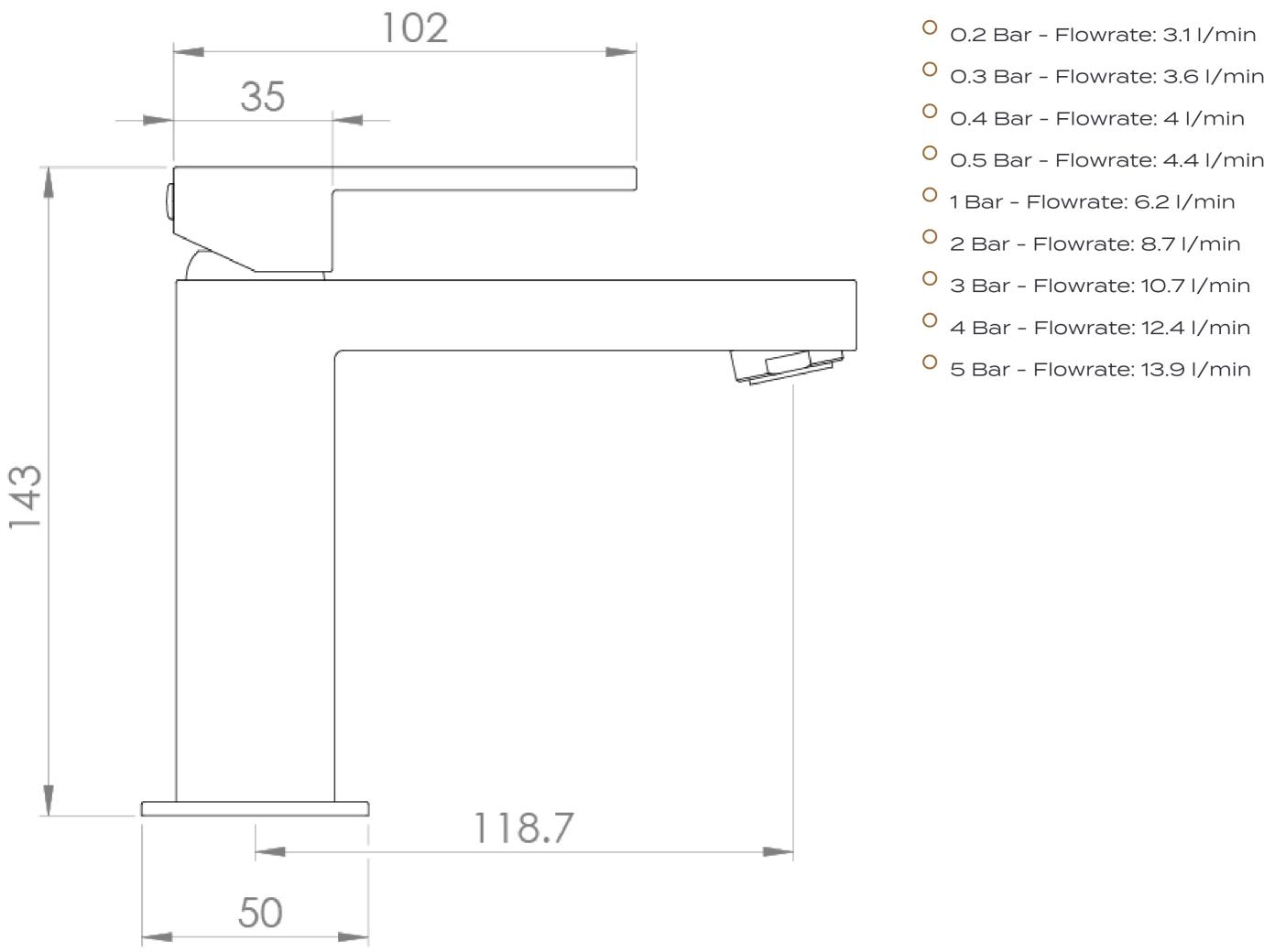
O.3 Bar - Flowrate: 3.6 I/min O.4 Bar - Flowrate: 4 I/min O.5 Bar - Flowrate: 4.4 I/min O 1 Bar - Flowrate: 6.2 I/min O 2 Bar - Flowrate: 8.7 I/min O 3 Bar - Flowrate: 10.7 I/min
